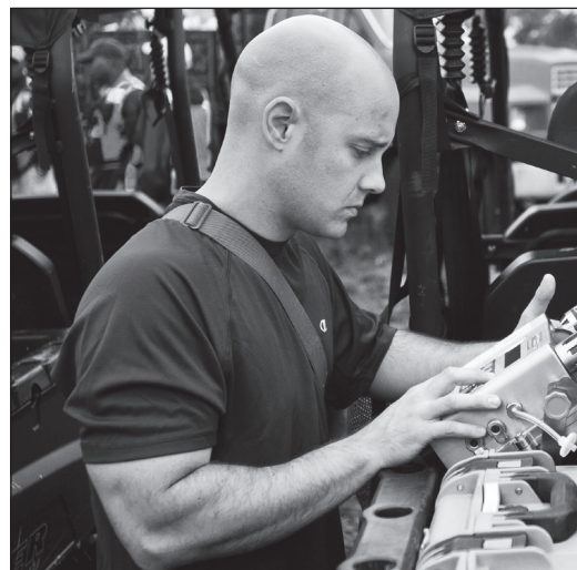
Below: Cloutier calibrates a remote air-monitoring device at the incident scene.
